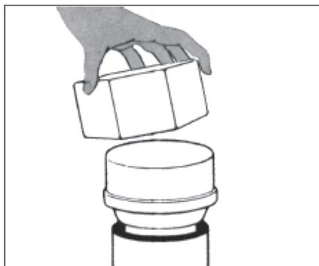
For installation in spaces with temperatures ranging between -40°F and 150°F. When installed in areas subject to extreme temperature conditions, the polystyrene package top should be fitted over the valve. When installing the Maxi-Vent® in outdoor installations a Maxi-Cap should be used to protect the Maxi-Vent from damaging UV Rays and extreme temperatures
